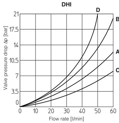
**7 OPERATING LIMITS** based on mineral oil ISO VG 46 at 50°C
